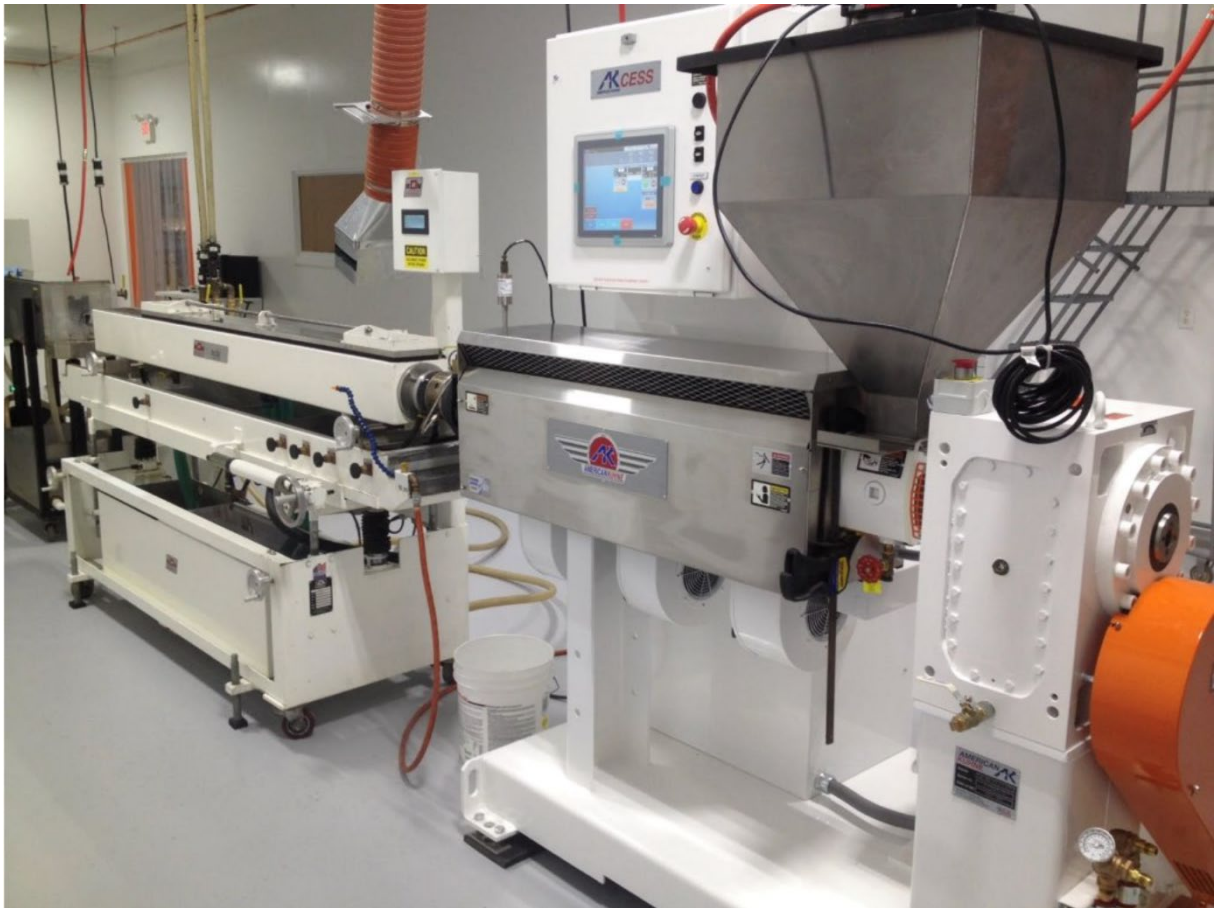
Fig. 1 Plastic extrusion machine [5]
